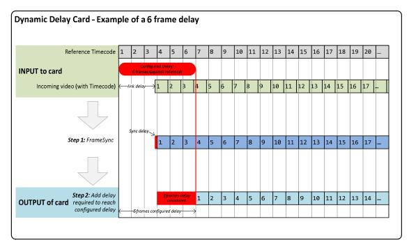
The card will work in both SD, HD and 3Gb/s mode. The input reference signal may not be in the same video format as the input video signal (but would have the same framerate), however both signals will include a SMPTE 12M-2 ANC VITC time code (Time of Day).
