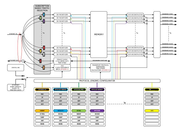
The modular structure of the ANCore enables to use the different engines for all different standards. A protocol (engine) configurator enables on the fly switching between the different standards and allows translation to and from different standards. Only the protocol unique and required parameters are set and influence the appropriate engine to do its job. This can be done for every stream individually.
