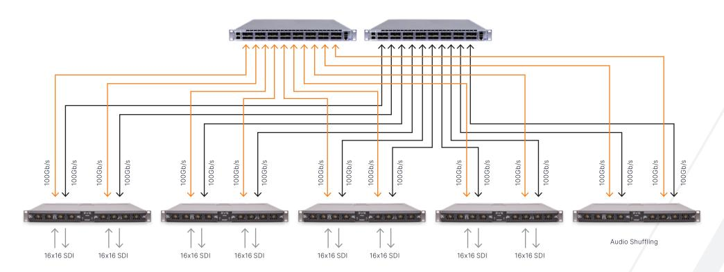
MediaInfra Strada-256 multi-level redundant system configured for 128x128 SDI with Audio Shuffling
