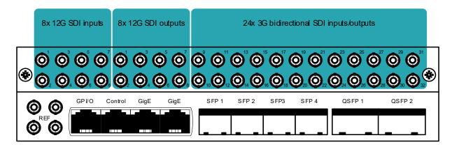
BRIDGE offers 32 x 1080p (= 8 x 2160p) processing paths in various configurations. Depending on the loaded configuration, some paths with include de-embedding and/or embedding. All paths include frame synchronization, audio gain/phase/delay processing, and color-correcting processing amplifiers.
